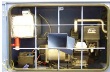
Fig. 2.6 APU and its extinguisher are protected with the grilles
